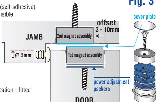
Note: to further reduce impact noise and bouncing effect when shutting door (especially when fitting the PLS24PRO to a double door set), also fit the Poron Xrd foam pad (supplied) to the door stop strip. (see the Poron info card inside the PLS24PRO package for fitting details).
